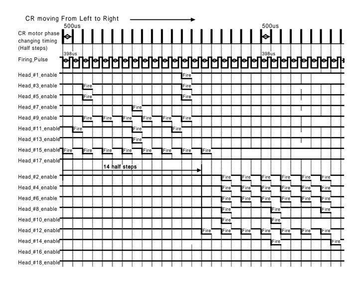
For Carriage moving right to left, timer for delay time dT should be added as same way of 1-2-3.
