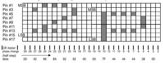
Expand the data to line buffer memory as below.
