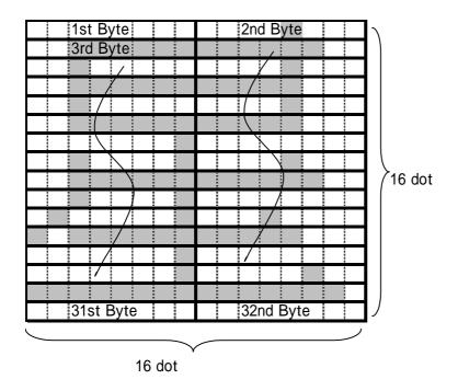
After reading these 32 bytes data, data structure should be changed to below order. "A" means odd pin printing data, "B" means even pin printing data. For example, 2A-7 is MSB of 2nd dot on odd pin pass, 2B-1 is LSB of 2nd dot on even dot. (2a-7,2A-6,2A-5,2A-4,2A-3,2A-2,2A-1,2A-0 is shown as 00000101.) 1A to 16A are 16 byte of odd pin data as 01 05 69 09 09 09 09 1F 09 09 0D E9 09 01 00. 1B to 16B are 16 byte of even pin data as 04 00 FC E4 E4 E4 E4 E4 E4 E4 E4 E4 FE 82 00 00.
