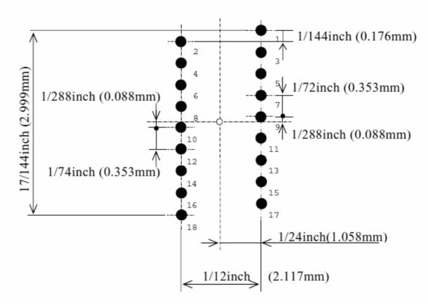
Above is the illustration of 18 pin print head. **Even number of pins are 14 half dot apart from odd number of pins horizontally**, and half dot apart from odd number of pins vertically.
