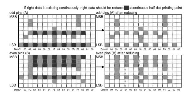
Finally, odd pins printing and even pins after 14 half dot moving. Each dot firing is same method as 1-2-2 and 1-2-3.
