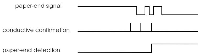
Figure 2-14 Paper-end detector operation
